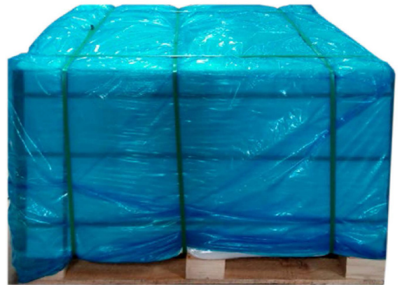
HARD CORRUGATED STRIP IS USED TO PROTECT PALLET CORNER ONLY EDGES OF PALLETS. SAFETY STRIP ON SIDES AND WRAPPED WITH BLUE STRONG PLASTIC CAP (9 MM).
