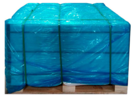
HARD CORRUGATED STRIP IS USED TO PROTECT PALLET CORNER ONLY EDGES OF PALLETS. SAFETY STRIP ON SIDES AND WRAPPED WITH BLUE STRONG PLASTIC CAP (9 MM).
